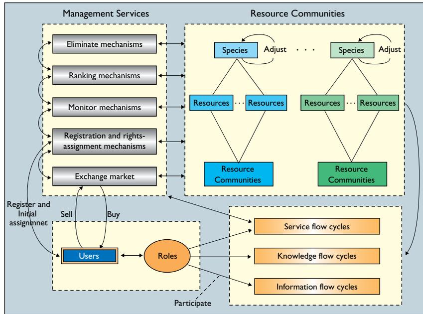
Figure 2. Eco-Grid architecture.
